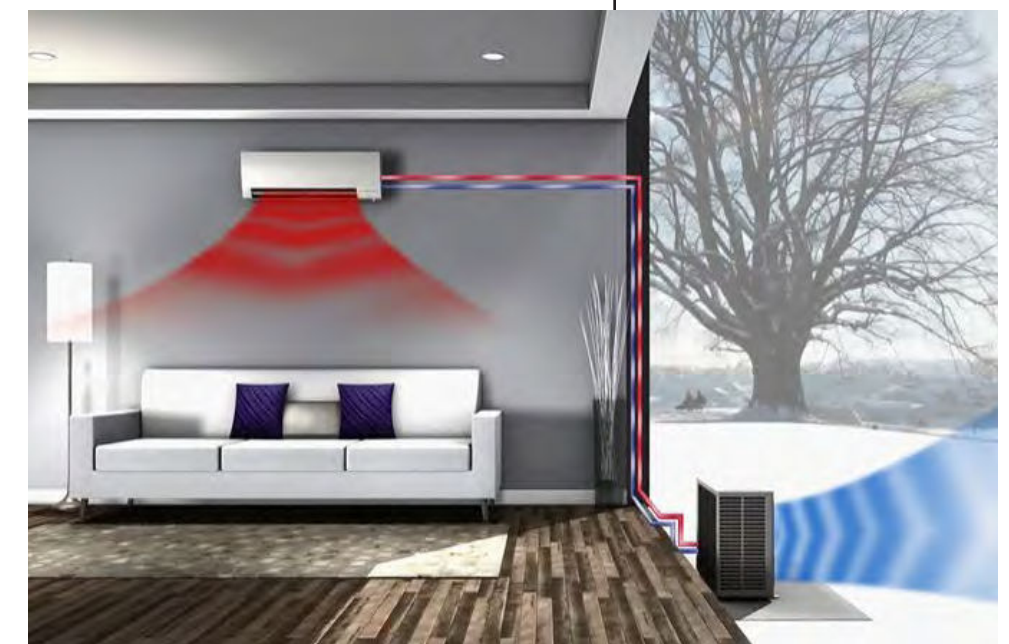
Diagram of the heat transfer between the outdoor unit and indoor unit during heating operation
